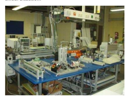
It is about a mechatronical production system where workpieces are transported on a band-conveyor to several stations (material detection and drill).
